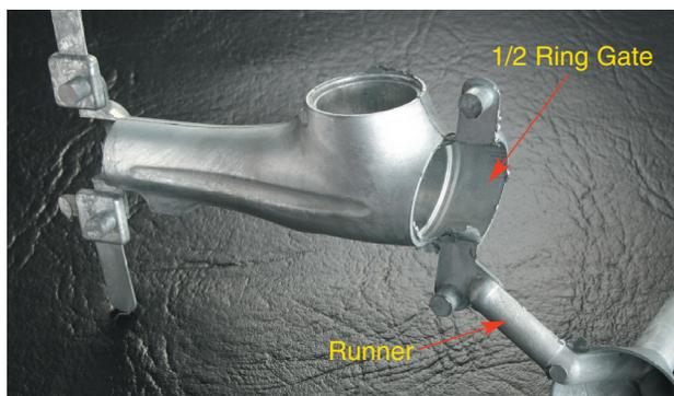
The overflows are positioned on the thin section end of the elbow furthest from the inlet gating. They also use a 1/2 ring geometry (with side tabs) on the thin end to avoid trim blemishes on the visible body of the elbow.
